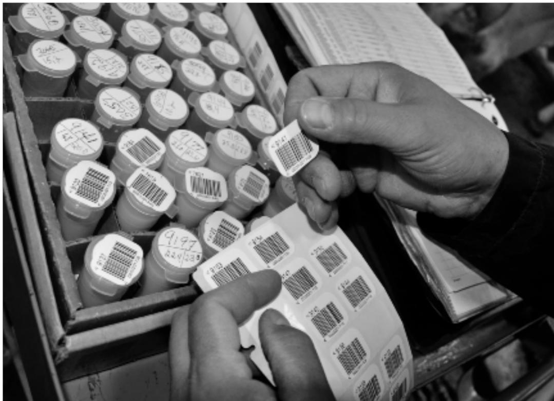
*The milk sample is collected at the farm and is placed in a 40ml test tube, identified by a unique bar code that includes the herd number and the cow number. It is then sent by DICOM to the Valacta laboratory in Sainte-Anne-de-Bellevue.*
